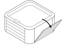
Open the side panel of your the Hot tub to access the unit control box
